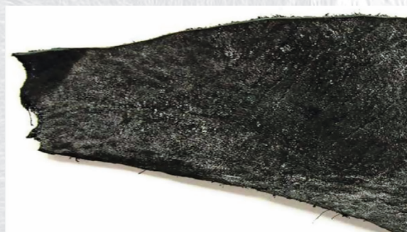
Fatty Spew (Minor Defective Area)
